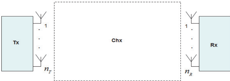
Figure 1. The MIMO system: conceptualization for the MIMO communication paradigm.
